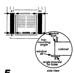
Place cabinet in window. Lower sash (window frame) to hold cabinet in place. Measure the distance between the side of the cabinet and inside of the window channel at the top and bottom of the cabinet. Adjust the cabinet until the distance on each side (top and bottom) is the same, so the cabinet is centered in the window. Write down the final measurement.
